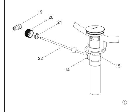
Remove the latch(19) and retaining nut(20). Fit the plastic washer(21) and retaining nut onto the ball lever(22). Insert the ball lever assembly into the drain lever hole and through the stopper hole. Tighten the retaining nut.
