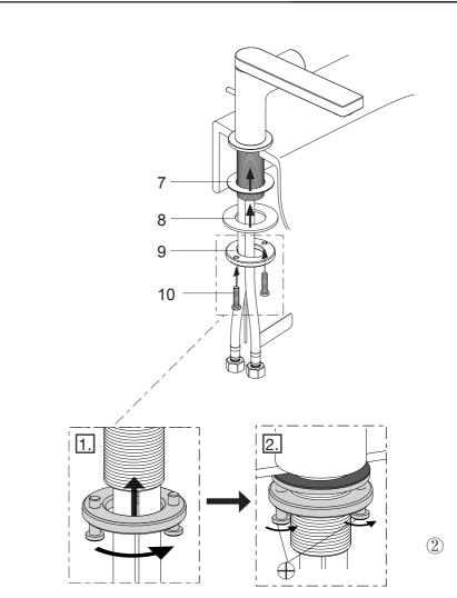
Position the faucet, install the screws(10) into the mounting nut(9). From underside of the lavatory, place the washers(7, 8) onto the shank. Tighten the mounting nut to secure the faucet. Tighten the screw.
